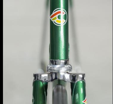
**TRADITION AND TECHNOLOGY** Columbus Spirit Super Pista tubes. Track fork with flat head and curved blades. Conical down tube improves lateral stiffness in the bottom
