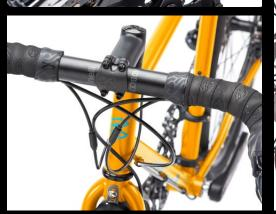
**COLUMBUS QUALITY** Columbus Cromor tubeset is the guarantee for quality, since 1919. The electrophoretic deposition process protects the frame from rust and corrosion and the double butted tubing ensure the proper thickness where necessary while being thinner – i.e. lighter – where no particular effort is needed.
